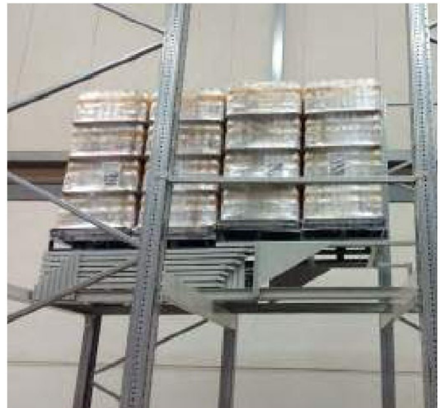
Convogliatore "lato 800 orizzontale" PUSH-BACK con pallet "DÜSSELDORF" PUSH-BACK conveyor with horizontal "DÜSSELDORF" pallets
