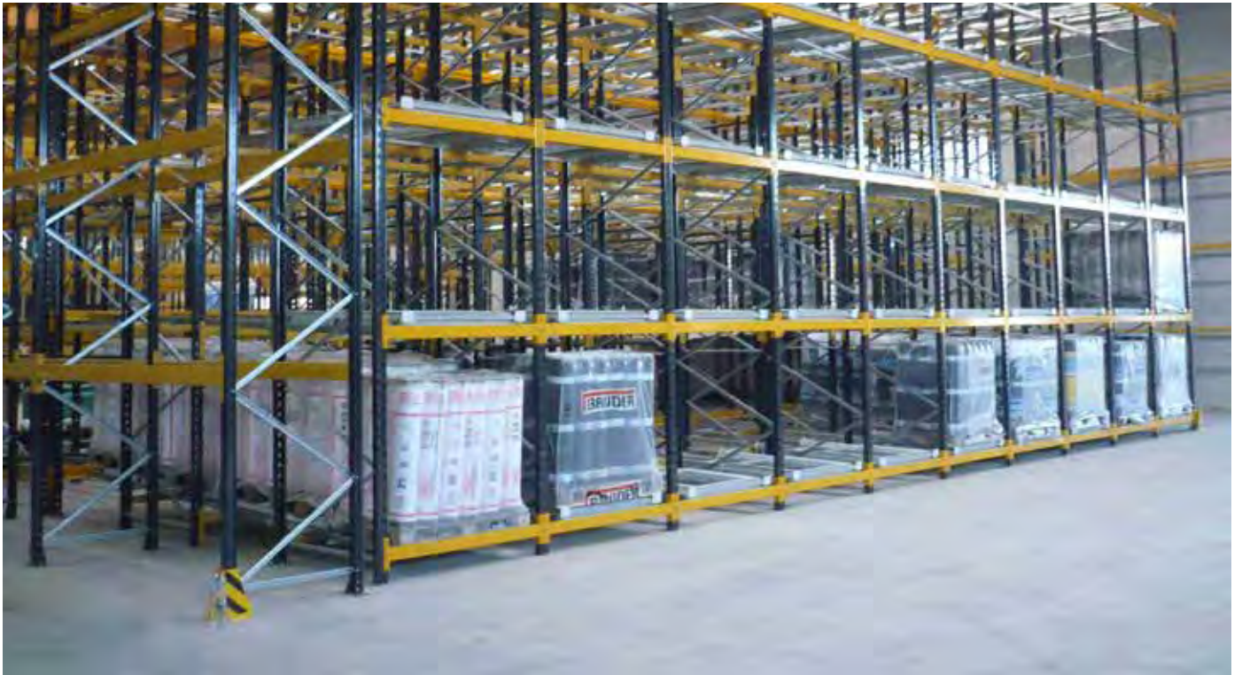
Magazzino in contropendenza LIFO attrezzato con moduli PUSH-BACK - LIFO warehouse with PUSH-BACK conveyors
