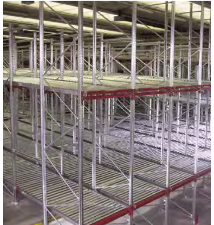
Magazzino LIFO / LIFO system
