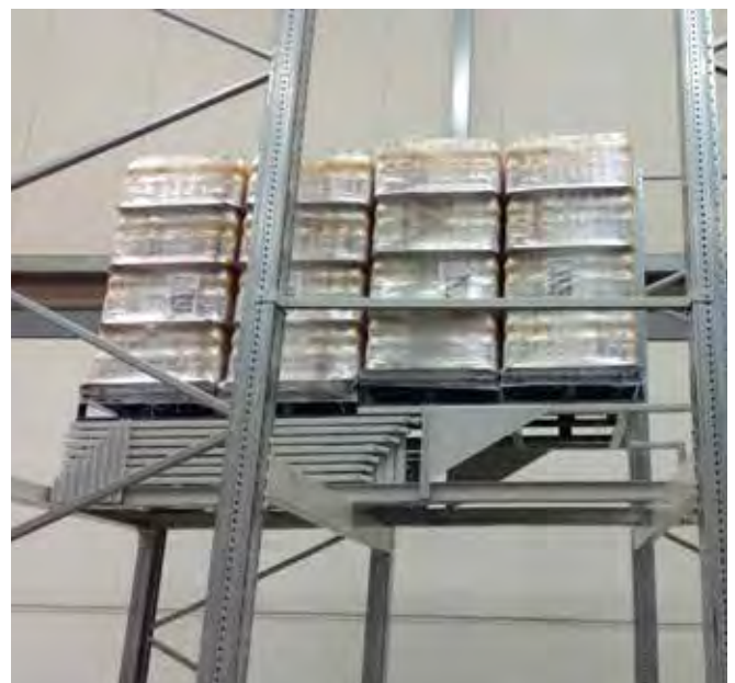
Convogliatore "lato 800 orizzontale" PUSH-BACK con pallet "DÜSSELDORF" PUSH-BACK conveyor with horizontal "DÜSSELDORF" pallets
